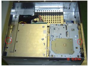
3. Remove four screws and take off HDD bracket.
